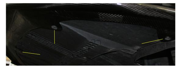
REMOVE ANY GLUE LEAKING IF PRESENT.
