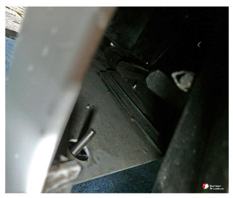
INSERT A M6 SELF-LOCKING NUT WITH WASHER AT LEAST 20 MM IN DIAMETER IN THE HOLE ON THE BUMPER.
