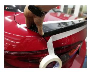
APPLY ACTIVATOR PRIMER ALONG THE PERIMETER WHERE WE ARE GOING TO APPLY THE DOUBLE SIDED TAPE, BOTH ON THE BOOT AND ON THE SPOILER (SEE PICTURE).
