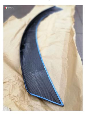
APPLY WINDSCREENS GLUE (OR EQUIVALENT, HIGH-ADHESION PROFESSIONAL ONE COMPONENT) IN THE FORM OF SCOOPS EVERY 15-20 CM INSIDE THE DOUBLE SIDED TAPE PERIMETER (SEE PICTURE).
