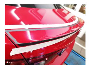
APPLY DOUBLE SIDED TAPE ALONG THE PERIMETER OF THE INTERNAL SURFACE OF THE SPOILER (SEE PICTURE).
