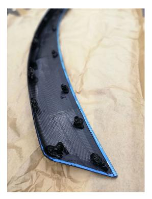
REMOVE THE PROTECTIVE FILM FROM THE DOUBLE SIDED TAPE AND PROCEED TO APPLY THE SPOILER ON THE BOOT, HELPING YOURSELF WITH THE PREVIOUSLY PLACED PAPER TAPE REFERENCES, STARTING TO BOND FROM ONE END OF THE SPOILER TO THE OTHER (DO NOT START FROM THE MIDDLE).
