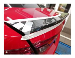
REMOVE EACH RETENTION TAPE OF THE SPOILER AFTER 24 HOURS, WHEN EVEN THE GLUE SCOOPS WILL BE DRY.
