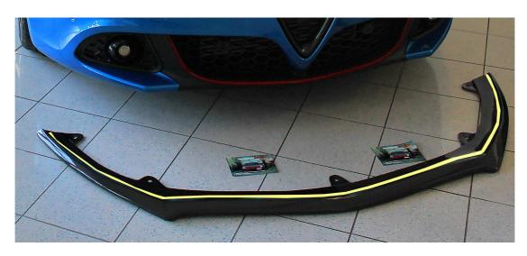
APPLY ACTIVATOR PRIMER ON THE AREA HIGHLIGHTED ON THE FRONT LIP, AS WELL AS ON THE BUMPER AREA WHERE THE GLUE WILL BOND.
