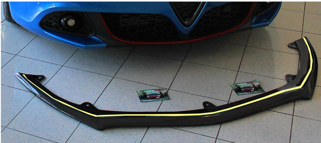
APPLY ACTIVATOR PRIMER ON THE AREA HIGHLIGHTED ON THE FRONT LIP, AS WELL AS ON THE BUMPER AREA WHERE THE GLUE WILL BOND.
