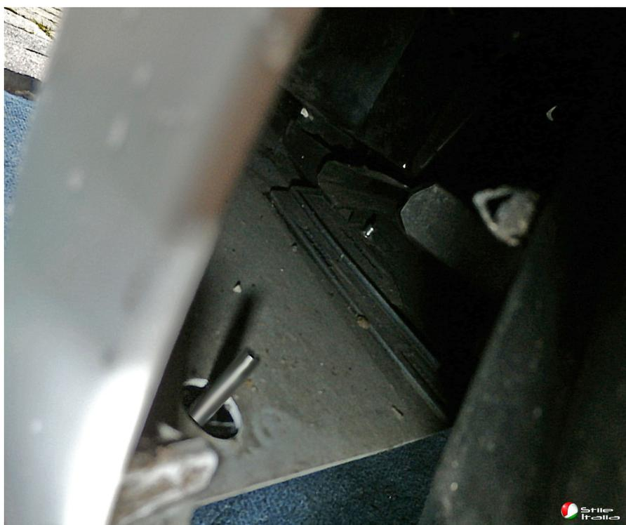
INSERT A M6 SELF-LOCKING NUT WITH WASHER AT LEAST 20 MM IN DIAMETER IN THE HOLE ON THE BUMPER.
